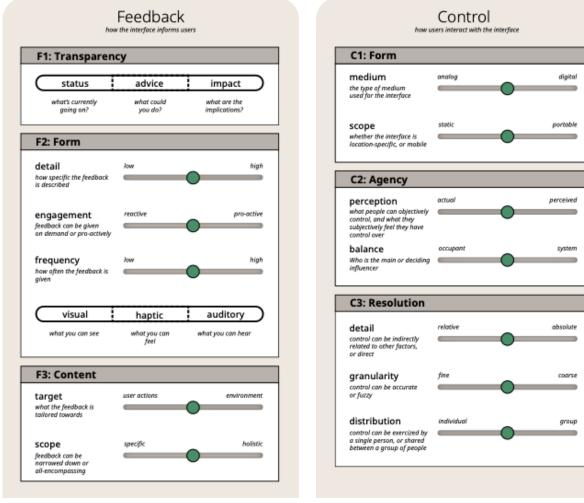
Figure 5: Design dimensions for interfaces
