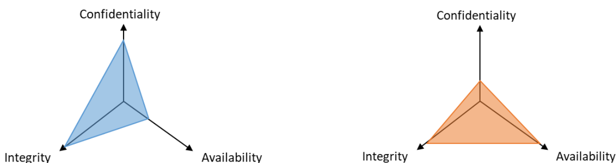
Figure 5: IT (left) prioritizes different elements of the CIA triad than OT (right)
