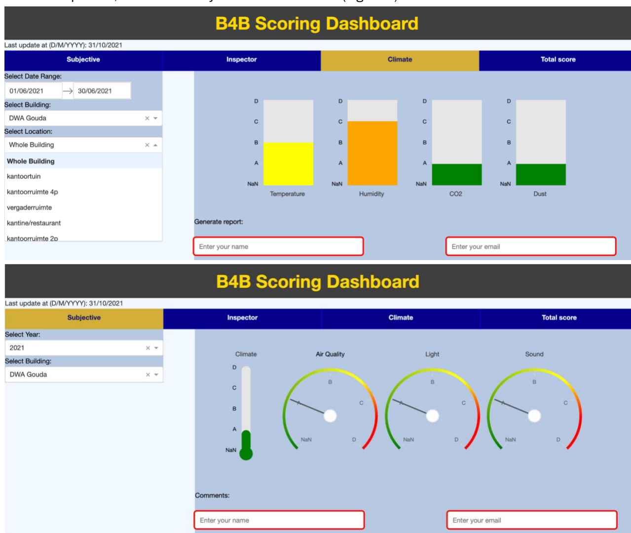
Figure 5: Two data dashboards were created for the B4B project connected to the data platform. The top figure shows the climate data for the entire DWA building. The lower figure shows the subjective comfort scores.
